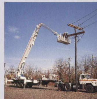
The first Bronto Skylift SI 155 with insulation was supplied to the USA, here serving a high voltage (500 kV) power line.
