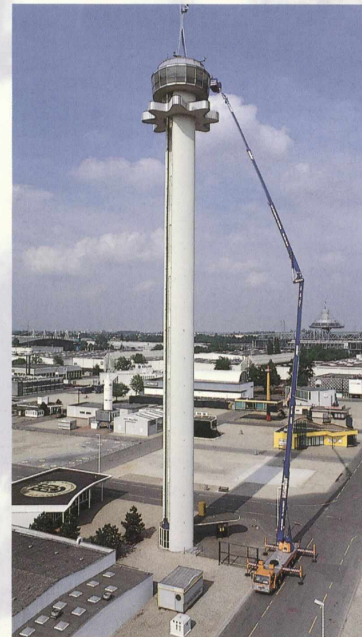
The world's highest industrial platform delivered to Germany, a Bronto Skylift S72 HLA, standing next to the Hermes Tower in Hannover.
