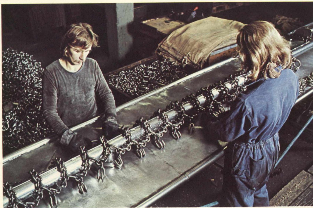
Final assembling of tractor chains at the Loimaa works.
