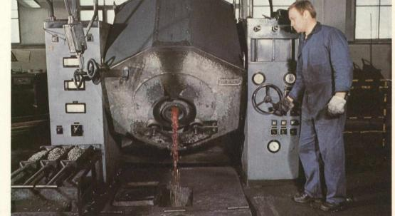
Supervising heat treatment of tapping screws at the Screw and fastening works.
