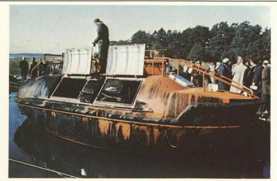
The Fiskars Survival 27, the life boat for ocean tankers, has just passed the fire test
