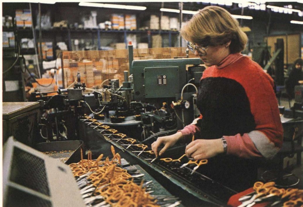
Sirpa Pulkkinen on the assembly line of the automatic scissors riveting machine at the Scissor Works.
