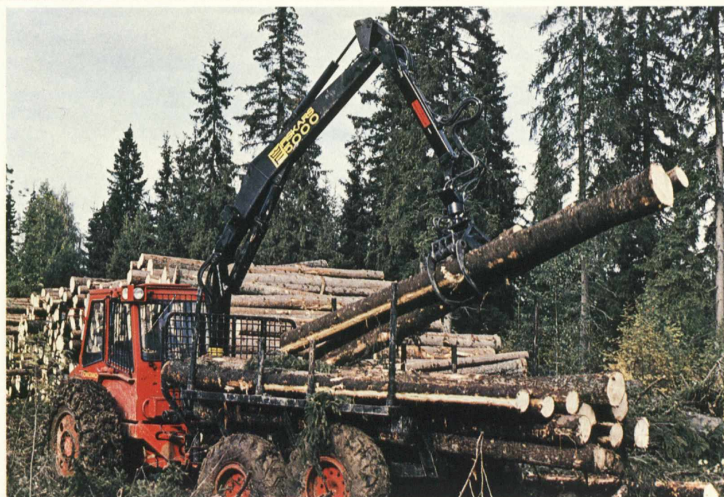
The F 5000 L hydraulic log crane, mounted on a tractor, brings a load of timber to be placed in temporary storage.
