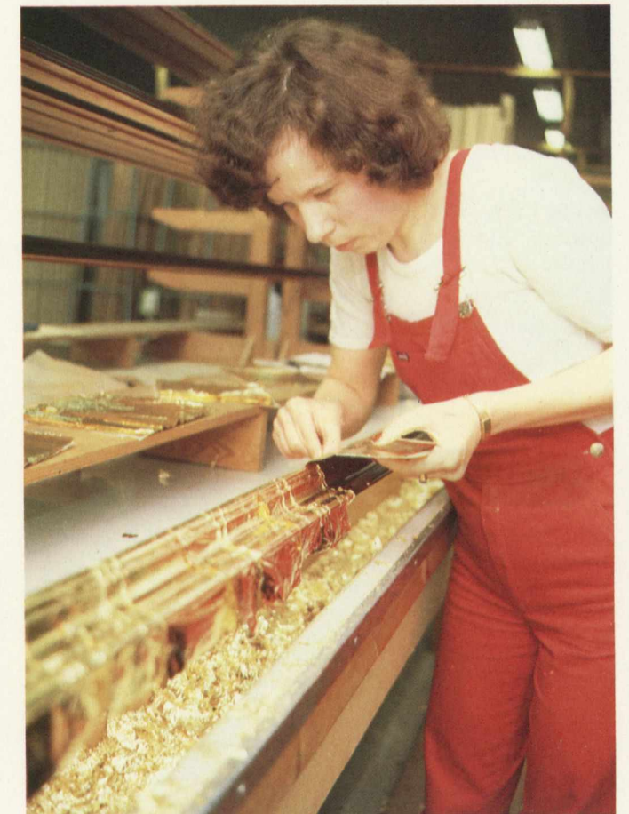
The majority of Fiskars picture frames are metallic plated in gold colour using machines, but for special commissions the work can be done by hand by the plant's skilled craftsmen.
